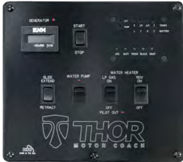
Typical Monitor Panel. Battery condition monitoring is usually located in the upper right corner.
