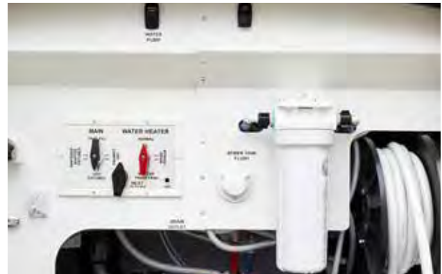
Illustrated here is a water system panel for a Class A motorhome. Features vary by model and floor plan.
