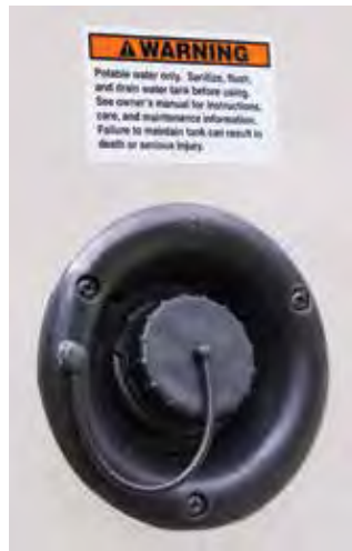
Typical fresh water gravity fill
