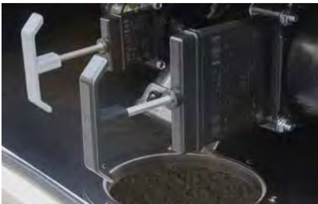
Typical termination valve configuration
