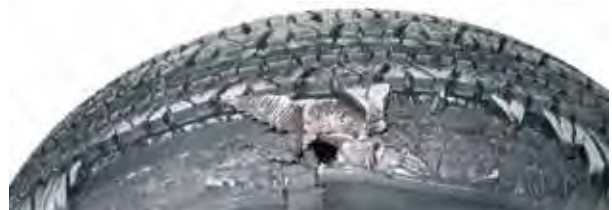
Tire pressure under and/or over inflation can cause serious tire failure
