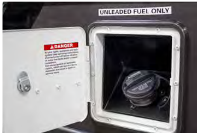
Fuel Tank Inlet for Fuel Transfer System
