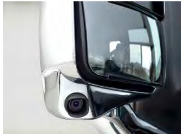
Mirrors are a vital component of safe motorhome operation. Convex mirror and side-view camera illustrated below.
