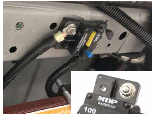
Typical 100 Amp Inverter Circuit Breaker located on a frame member underneath the vehicle, near the battery trays.
