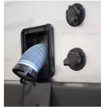
City water fill connection, along with a storage chamber for the sewer hose. This image for reference only. The water ports on Class B motorhomes vary in type and location due to floor plans and features.
