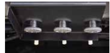
Low point drain valves are typically located underneath the left-side rocker panel
