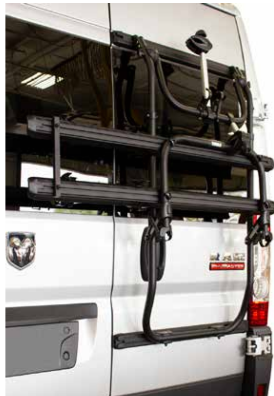
Bicycle rack attached to the rear door
