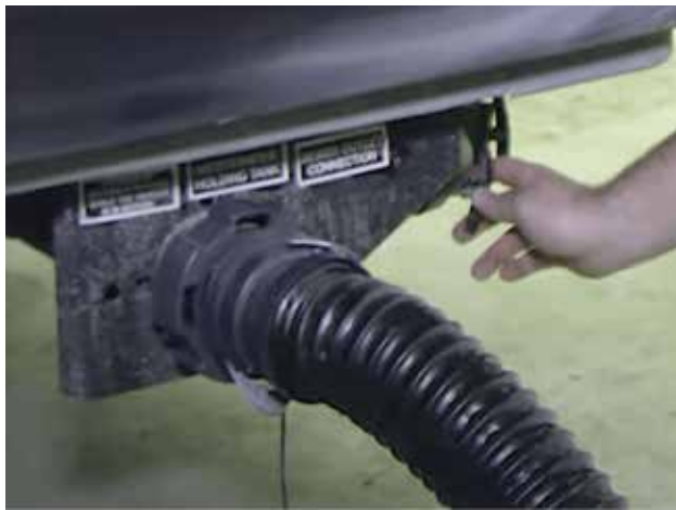
Location of Termination valves is typically on the left side of the motorhome. Class B camper-vans with cassette toilets will not be equipped with a black wastewater termination valve.
