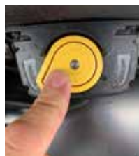
Safety Relay rotated to the ON position. Depress the center to engage the safety relay
