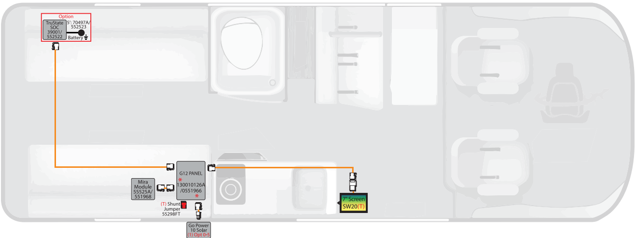
Wiring illustration (above) of a typical Firefly multiplex system; consisting of main touchscreen control panel, wireless room switches, and main electrical control board.
