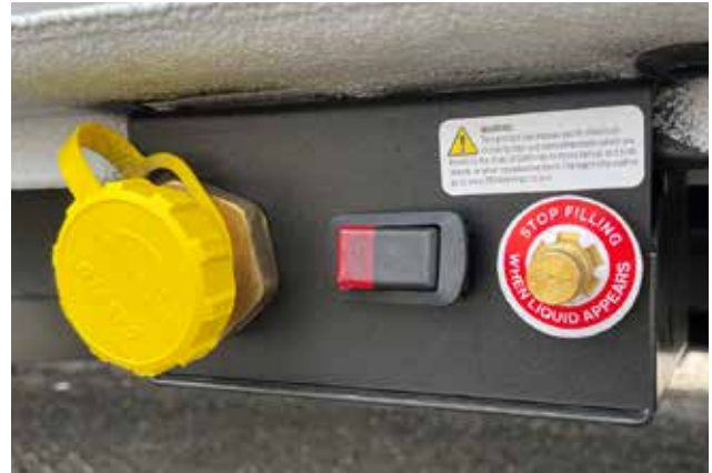
Propane access panel, positioned along the lower left side of the vehicle
