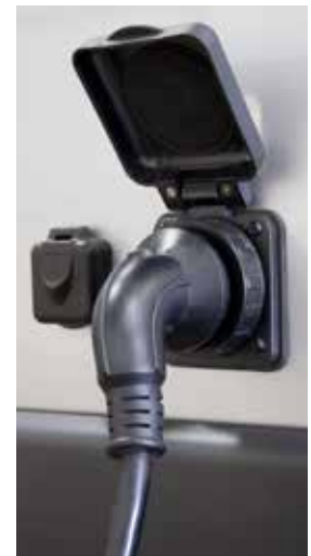
Typical shoreline power cord connection port
