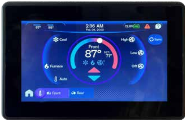
Set the desired air conditioned temperature from the Climate Menu on the Multiplex Touchscreen Controller.
