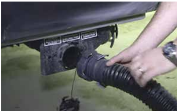
Typical sewer hose connection. Slip hose onto outlet and twist to lock.
