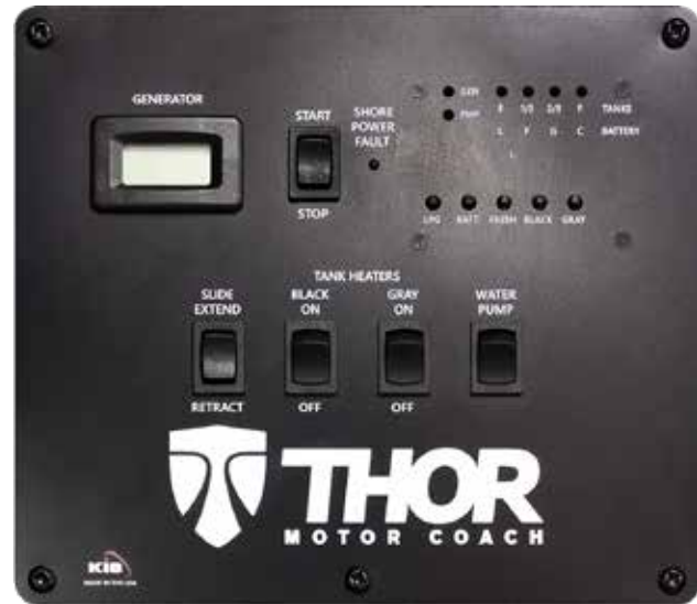
Typical Monitor Panel
