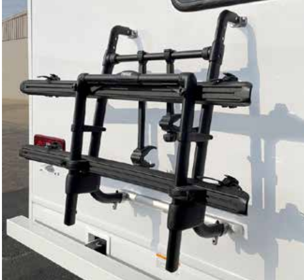
Typical bicycle rack installation
