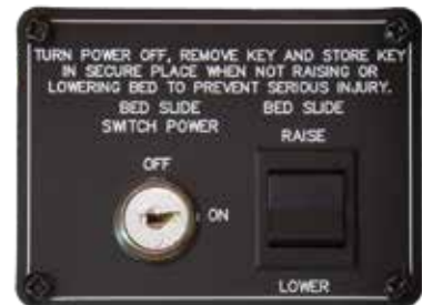
Figure 3. With multiplex systems, the powered over-cab bunk operating controls are usually located on the Slides/Awnings Menu. Some multiplex systems will also include bunk controls on a convenient wall switch.
