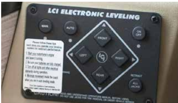
Typical Leveling Control Panels (above), which may contain an LCD read-out. Hydraulic pump assembly (below)
