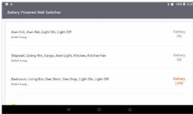
Battery powered wall switches settings. LOW indicates that the battery in the wall switch needs replacing.
