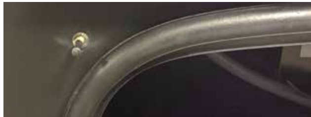
Fuel Pump Safety Lock-out Switch
