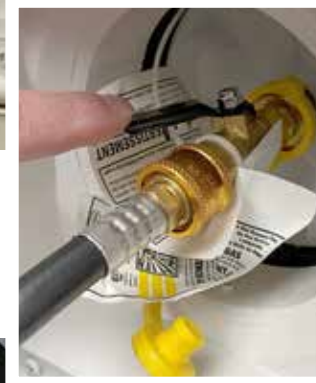
(Above) Typical external propane hook-up port. (Right) manual shut-off valve.
