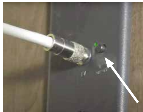
Antenna/Cable push-button selection switch with green LED
