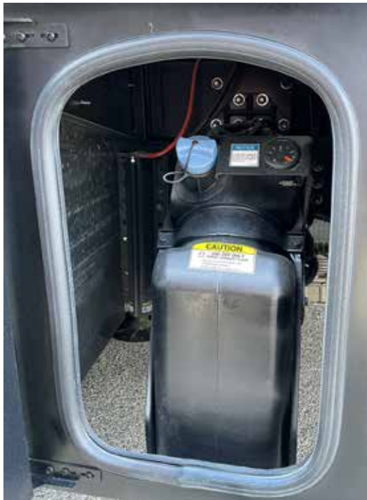
Typical DEF tank.
