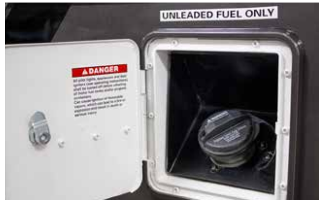
Fuel Tank Inlet for Fuel Transfer System
