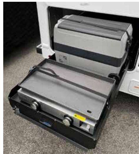
Portable LP Griddle and 12 volt cooler mounted on a rearward slideout tray.
