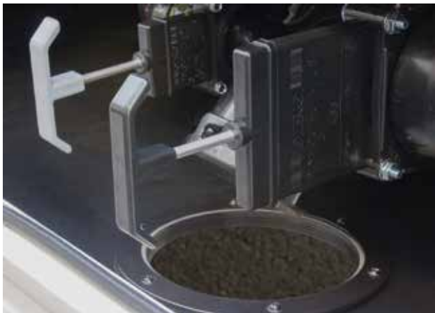
Typical termination valve configuration
