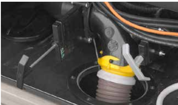
Black tank termination valve in the OPEN position.
